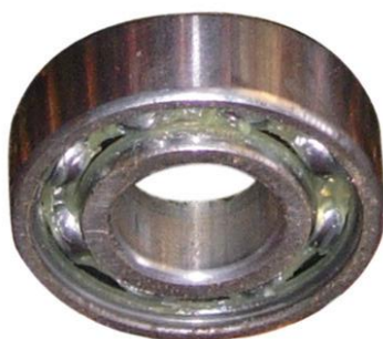
Fig. 12.16 : Ball bearings reduce friction
