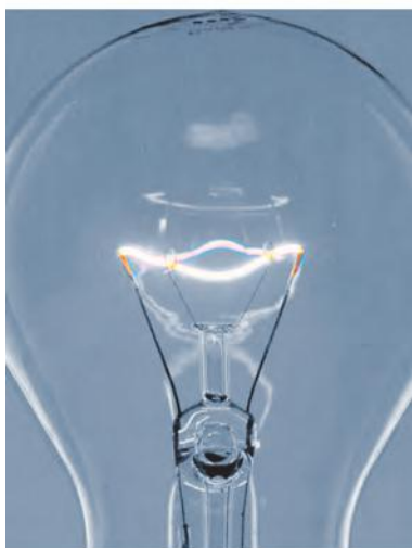
Fig. 14.12 Glowing filament of an electric bulb (incandescent)
