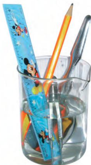
Fig. 4.8 Conduction of heat by different materials
