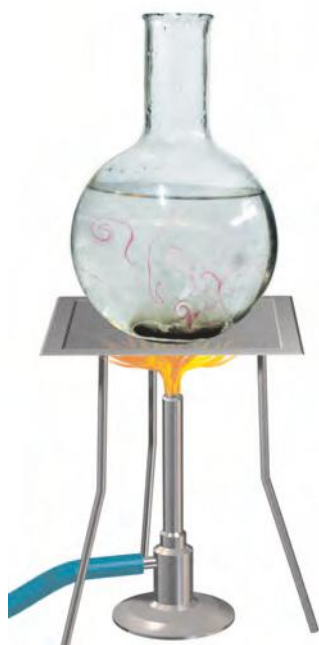
Fig. 4.9 Convection of heat in water
