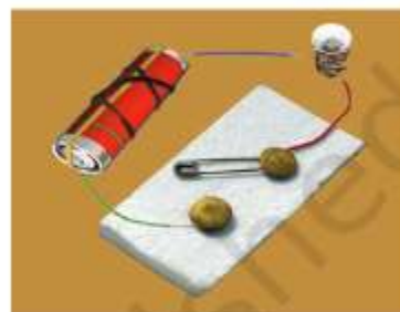
Fig 12.9 An electric circuit with a switch
