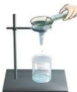
Fig. 5.10 Filtration using a filter paper
